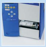
The dispensing unit separates the label from the carrier and provides it for further processing. After removing the label, another print order is activated by the dispensing photocell or an external impulse.
